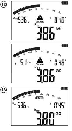
View of the screen during measurement. The LOCK means that the measurement was started with ENTER button or by pressing and holding START button for approx. 5 sec.
