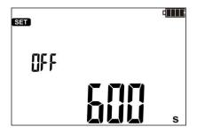
Use buttons and to set Auto-OFF time or to inactivate this function (horizontal lines – Auto-OFF function is inactive). Auto-OFF function is used to turn-off inactive meter after a preselected time (300, 600 or 900 sec.). When the user switches the meter off, it will generate a beep after the set time.
