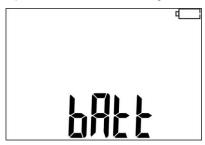
The battery pack is fully discharged,
