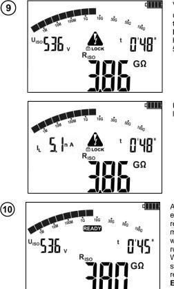
View of the screen during measurement. CLOCK means that the measurement was started with **ENTER** button or by pressing and holding START button for approx. 5 sec.
