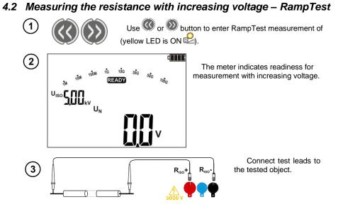
Use **SET/SEL** button to enter the settings of the measuring voltage  $U_{\text{ISO}}$  and measurement duration settings.
